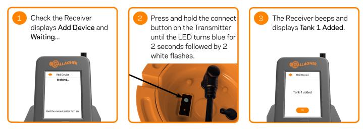
Repeat the above procedure if adding additional Data Transmitters. Gallagher recommends configuring all Transmitters prior to physical installation.
