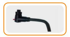
**Important:** Manually bend the cable **PRIOR** to connecting the sensor cable to the Transmitter. If the cable is bent once connected to the Transmitter the waterproof connector may be damaged. Refer to the photograph for the correct technique.
